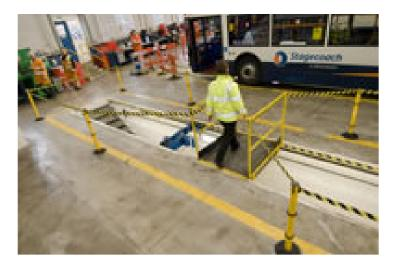
**Other types of barrier:** Guard rails, chains or extendible barriers can provide protection for workers near the pit edge. They allow access to the side of a vehicle over a pit (as the vehicle covers the pit at this point) while providing a warning of the open pit not covered by the vehicle. They need to be sufficiently high, stable and clearly visible so that they do not create a tripping hazard.
