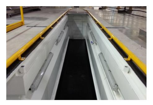
**Reducing the risk of slips and trips:** Ensure the surface around the pit is slip-resistant, either by using anti-slip materials or by having an effective cleaning regime. As far as possible, keep the area clear from obstructions and deal with spills immediately. Similarly, keep the area inside the pit free from obstructions, this will improve access for pit workers.
